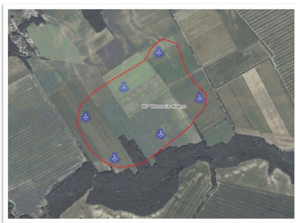
Figure 5 Locations of WTG's (marked with blue icon) in the Wrzeście-Kępno subproject, approximated WF border is marked with red line
